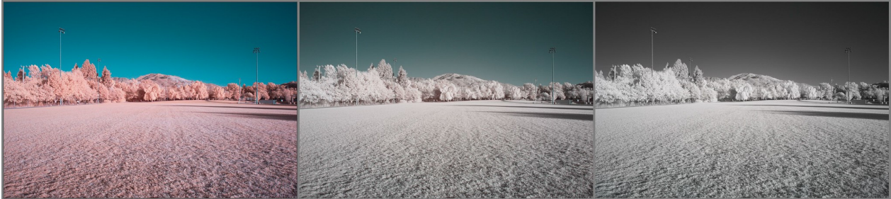
The same scene with three different infrared filters: 590nm, 720nm, 850nm.
