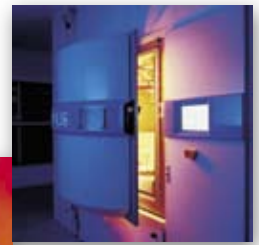
In ultra-modern vacuum coating facilities, a reflex-reducing layer is applied
